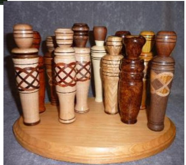
John starts the call with a 2 x 2 block of wood and drills a 5/8 inch hole. "The barrel gives the maker his own 'style'". John did little turning at the demo, mainly, he talked the group through the process of making the call. John buys his call supplies, such as Mylar sheets to use as the "reed", from Hut Products ( [www.hutproducts.com](http://www.hutproducts.com) ).
